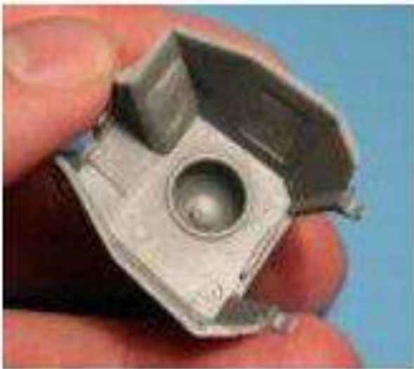
Ejection Pin Marks
